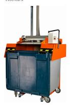
The safety system ensures, among other things, that bins of different sizes are installed correctly before the machine can be operated.
